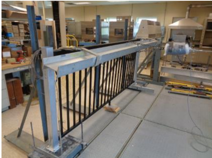
Photo No. 5 Horizontal Concentrated Load on Top Rail Adjacent to End Post
